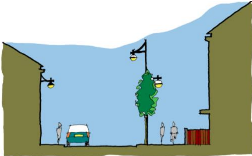
Diagram showing a section through a major access road with widened footway with cycle way on one side.
